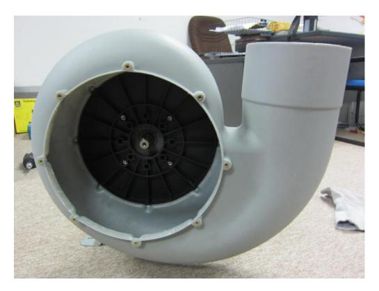
4. Install the PP impeller on the motor with impeller assembly screw.
