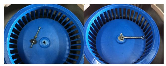
5. Tighten the PP impeller with screw provided.
