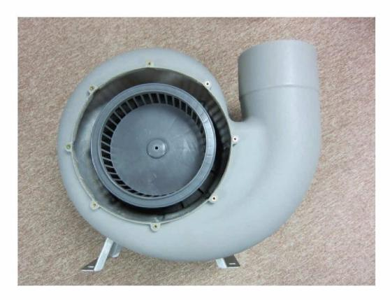
4. Install the PP impeller on the motor.
