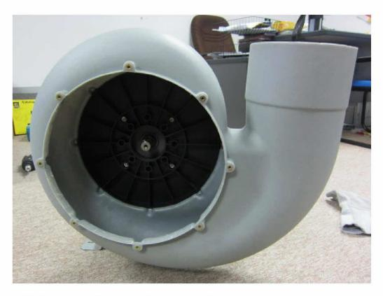
3. Install fan easing on the motor with screws provided.
