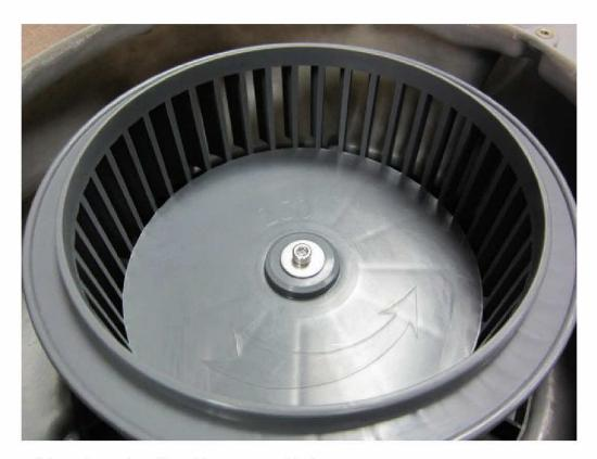
5. Tighten the PP impeller with screw provided.
