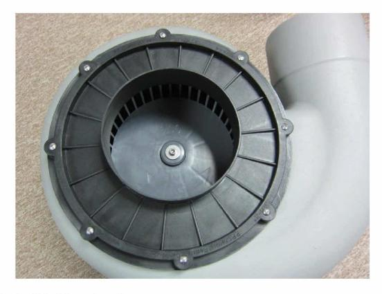
6. Install fan inlet on the casing.
