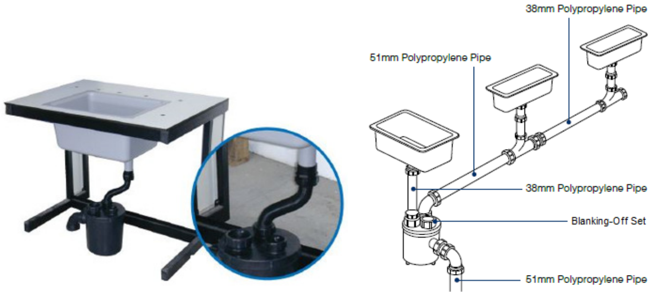
A typical laboratory bench waste run incorporating sinks discharging into a catchpot.
